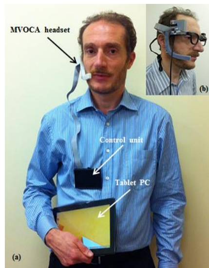
Fig. 4. Two MVOCA headset designs, a) mounted on a headband and b) attached on a pair of glasses. Appearance of the devices when worn by a user.
