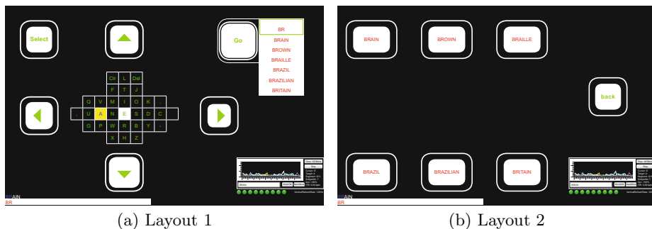
Fig. 2. GUI of the dictionary-driven SSVEP-based Speller with a modified GUI. After spelling two letters, up to six words to choose from are suggested on the right side of the button “Go”. If the desired word is amongst those, as it is shown in Fig. 2 (a), the BCI user can switch to layout 2 by means of the “Go” command. In layout 2 (shown in the Fig. 2 (b)) the whole word can be written by selecting the corresponding flickering box. In case of erroneously selecting the “Go” command, the user can switch back to layout 1 with the “back” command.
