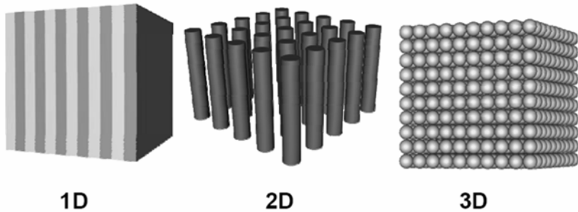
Fig. 1. Examples of one- (1D), two- (2D), and three-dimensional (3D) photonic crystals. The main feature of a photonic crystal is the periodicity of dielectric materials along different axes.
