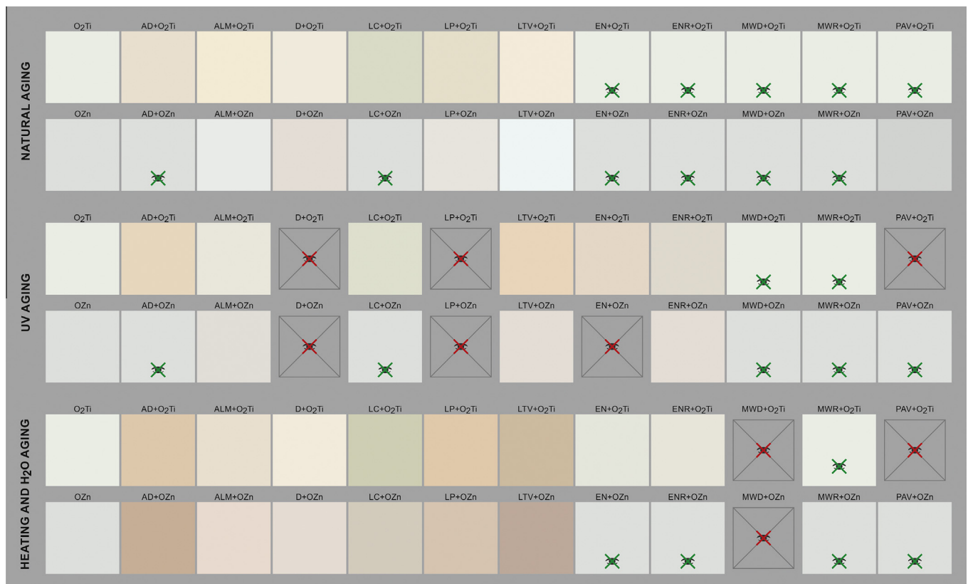
Fig. 6. Simulated colour card using the software Spectra Magic de Konica Minolta. The first colour in each series corresponds to the pure pigment. It is followed by colour simulations with the different techniques. Symbol of the eye crossed out in green = samples with variations unrecognizable to the human eye. Symbol of the eye crossed out in red = samples not measured for deterioration. (For interpretation of the references to colour in this figure legend, the reader is referred to the web version of this article.)
