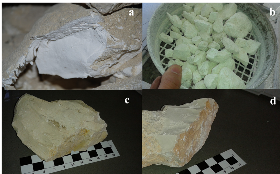
Fig. 2. a) Quicklime (TL) obtained by traditional process. b) Quicklime (IL) obtained by industrial process. c) limestone from Gilena quarry d) limestone from Morón de la Frontera quarry.
