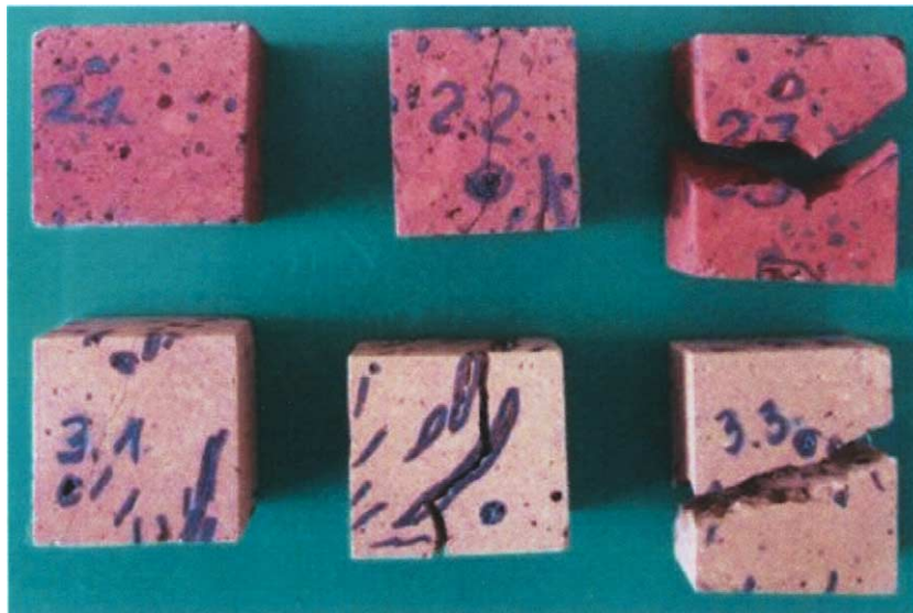
Fig. 8. Appearance of some red and yellow bricks after freeze–thaw test. Samples that have withstood under accelerated aging test can be distinguished from those totally broken. (For interpretation of the references to colour in this figure legend, the reader is referred to the web version of this article.)
