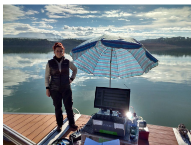
Elizabeth León-Palmero, researcher in the Department of Ecology, University of Granada, with the device that enables researchers to measure the CO 2 , CH 4 , and N 2 O flows simultaneously (PICARRO).
