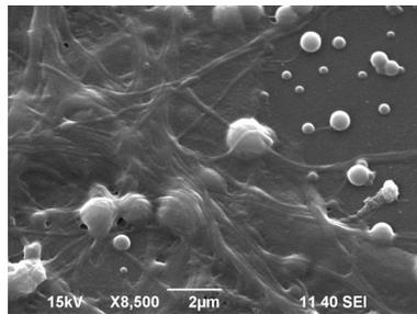
*Scanning electron microscopy image showing detail of the neural network on a layer of nanoparticles.*
