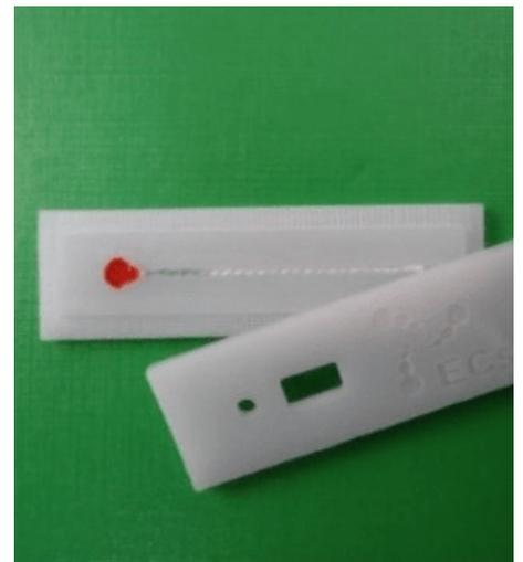
on cotton thread combined with a smartphone to photograph the device, analyse the colour produced in the testing, and calculate the concentration. For example, the concentration of potassium in water, of creatinine in urine, or of glucose in blood can be calculated by adding just a tiny volume of the relevant sample into the device, which provides the results in seconds.
