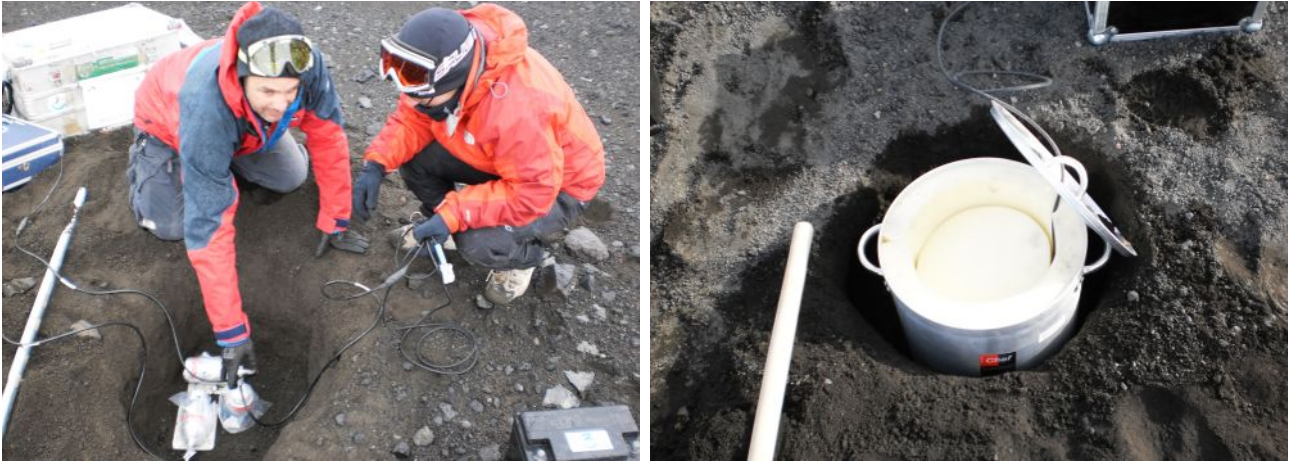
Figure 7. Left: installation of a three-component Mark Products L4C seismometer; right: installation of a three-component Lennartz 3D/5s seismometer.
