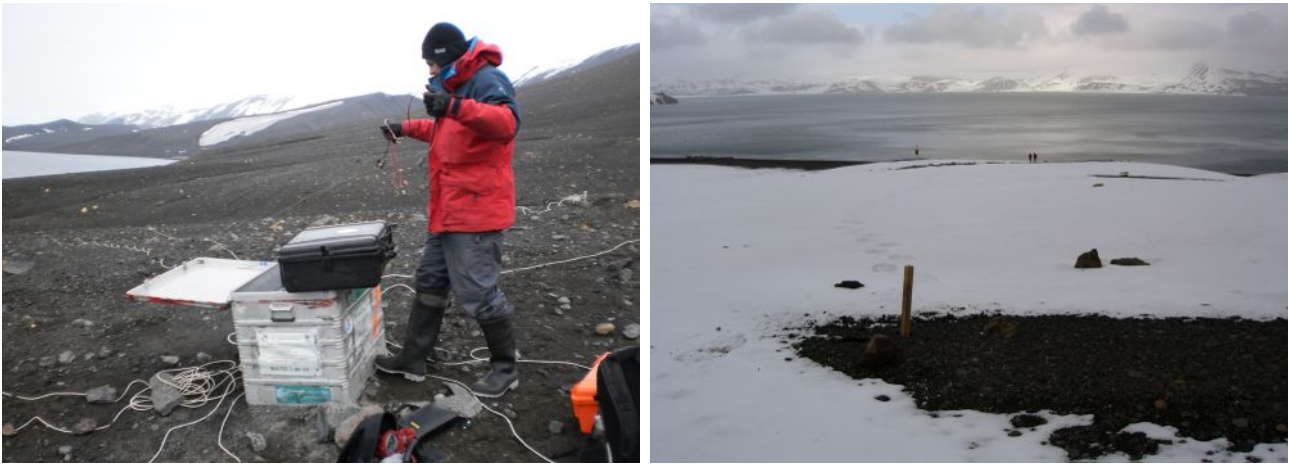
Figure 9. Left: installation of the array data acquisition system in the Fumarole Bay area during the 2010-2011 survey; right: reference stake indicating the position of one of the seismometers of the 12-channel seismic array deployed in the Fumarole Bay during the 2009-2010 survey.
