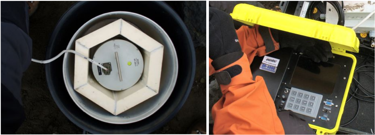
Figure 12. Seismometer (left) and data acquisition system (right) of the permanent station DCP, installed in February 2008 at Deception Island.
