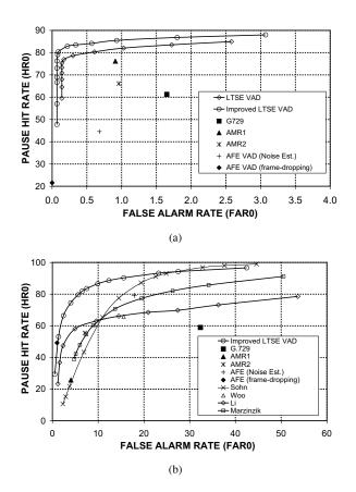
Fig. 2. ROC curves. (a) Close talking microphone (stopped car, motor running). (b) Distant microphone (high speed, good road).
