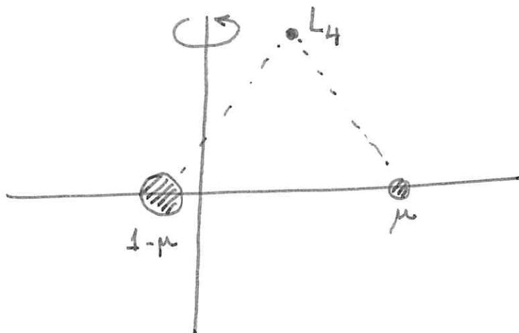
The primaries have masses  $1-\mu$  and  $\mu$  with  $\mu \in [0, \frac{1}{2}]$ . The whole plane is rotating around the vertical axis and the satellite is placed at the vertex of an equilateral triangle composed by the three bodies. Note that in the rotating system  $L_4$  is an equilibrium but in the inertial system it is a periodic solution. In this case the periodic solution is known explicitly and the linearized system is autonomous.
