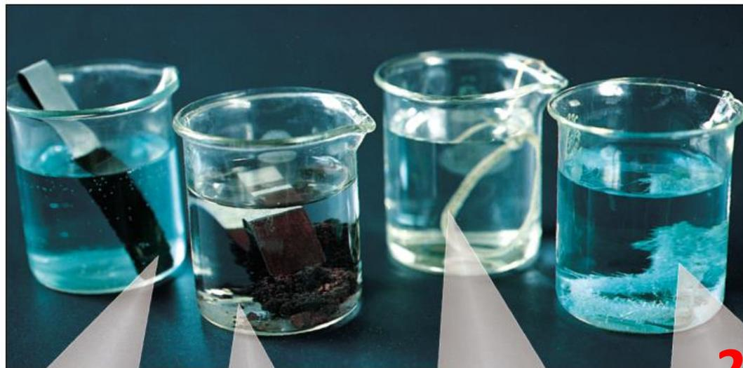
The Zn bar is in aqueous solution of  $\text{CuSO}_4$
