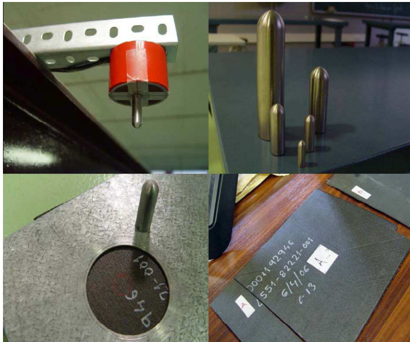
Fig. 1. Impactors and specimens used in the experiments.
