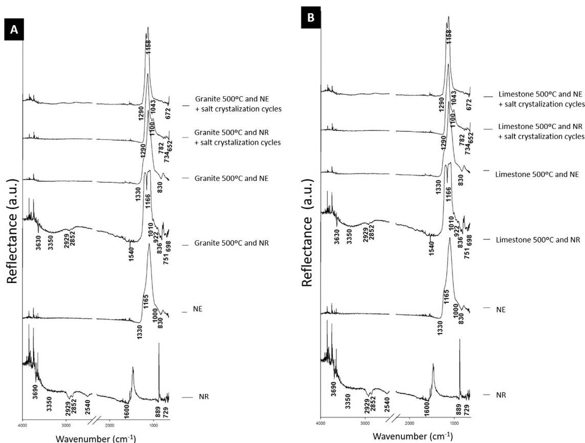
Fig. 6. FTIR (reflectance) spectra collected on nanoconsolidants powder, the stones consolidated and the coated samples after fourteen salt crystallization cycles. A: Granite samples. B: Limestone samples. NE: Nano Estel® and NR: Nanorestore®.
