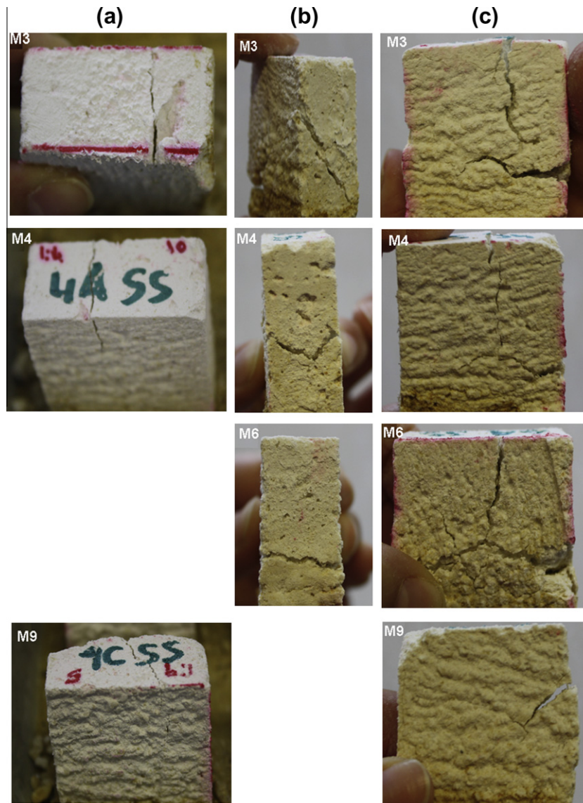
Fig. 4. Images of the different deterioration forms appeared in the mortars samples submitted to the WS + SS test (weathering study and salt resistance by capillary absorption): (a) Fissures developed after four cycles in samples M3, M4 and M9. (b) Efflorescences appeared after six cycles on the side surfaces of samples M3, M4 and M6; spalling also appears on sample M9. (c) Fractures in form of cross developed in all samples after six cycles.
