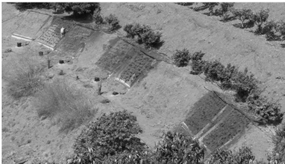
Fig. 2. Closed erosion plots in the taluses of orchard terraces with the different plant covers.
