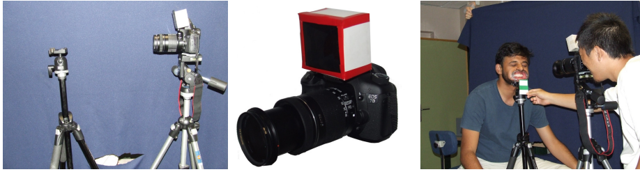
Fig. 1. Experimental set-up and image acquisition: basic scene set-up (1), camera with polarization filters (2), image acquisition (3)
